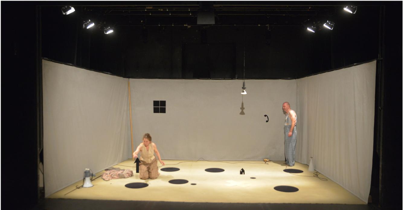
Material of our curtain hardly inflammable in accordance with DIN 4102 B1
